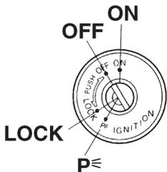
The main switch/steering lock controls the ignition and lighting systems, and is used to lock the steering.
