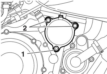
1. Engine oil filter element drain bolt
