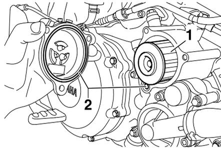
1. Engine oil filter element
