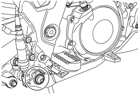
The operation of the brake pedal should be checked before each ride, and the pedal pivot should be lubricated if necessary.
