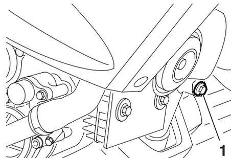
1. Engine oil tank drain bolt
