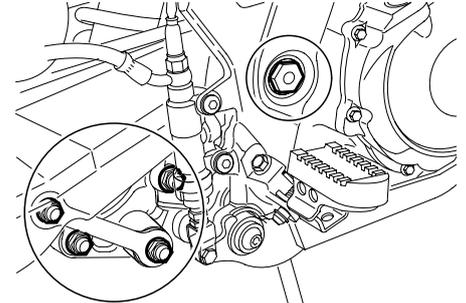
The pivoting points of the rear suspension must be lubricated at the intervals specified in the periodic maintenance and lubrication chart.
