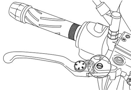
The operation of the brake and clutch levers should be checked before each ride, and the lever pivots should be lubricated if necessary.
